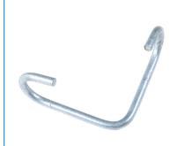
The 90 Degree S-Hook is used to hook wire tensioners, heavy duty springs and strain insulators onto the Omega end and corner brackets and allows a tensioning point in corners. The 90 Degree S-Hook can also be used to split zones in corners.
