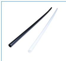
Stay sleeves insulate the stays from live fence wires and protect the wires from arcing onto the stay and causing false alarms. Available for the 8mm or 10mm stay.
