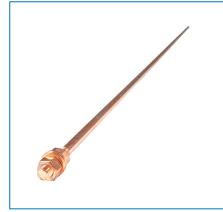
The copper cladded earth spike or stake is used to earth the electric fence system. A minimum of 3 earth spikes must be knock into the ground near the electric fence at a minimum of 1.2m apart. Connect these earth spikes to the energizer or the fence using the high tension insulated cable (HT). In areas where earthing conditions are bad you may be required to add a few more earth spikes/stakes along the fence line and connect these back to the energiser.
