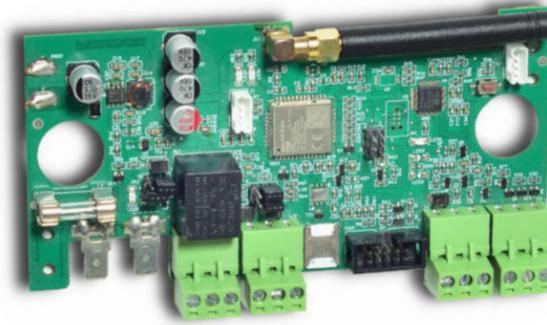
Nemtek Connect works by connecting to a Nemtek electric fence energizer with GSM cellular connectivity via a GSM module. This module allows the energizer to communicate with the mobile application, providing real-time updates and control over the electric fence system. Users can access the mobile application from a smartphone or tablet with access to a GSM cellular network, allowing them to remotely monitor and control the electric fence system from anywhere with an internet connection.
